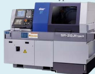
CNC Swiss Type Automatic Lathe
