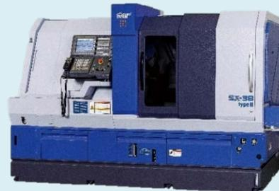
CNC Swiss Type Automatic Lathe
