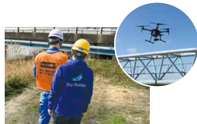
Water pipe bridge inspection using drones
