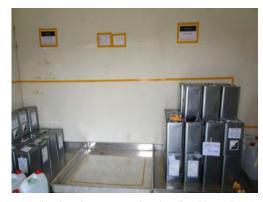
A yellow line drawn to visualize the allowable stacking height of containers in a hazardous material storage area
