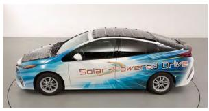
Prius PHV demo model equipped with solar battery panel
