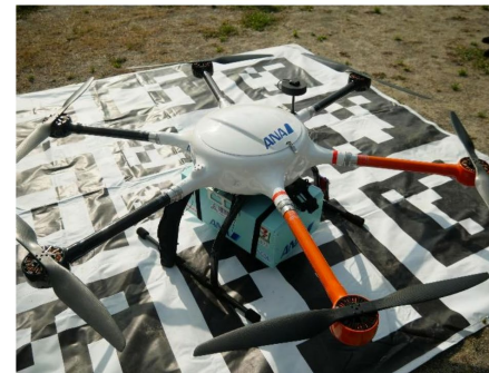
5 kg payload delivery drone prototype
