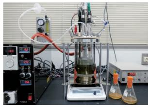
Ethylene production equipment (electrified cultivation equipment)
