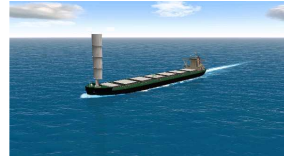
The coal carrier equipped with a hard sail wind power propulsion system known as “Wind Challenger” to start operations in fiscal 2022.
