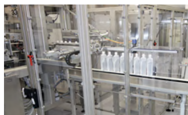
Newly added BFS (Blow Fill Seal) line at SterRx facility
