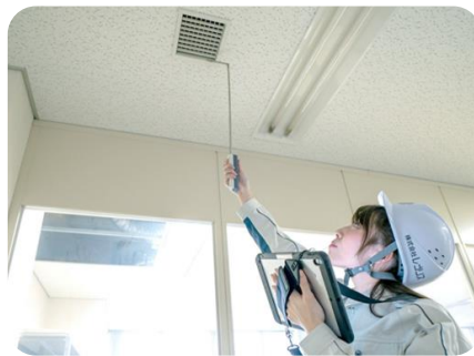
Airflow measurement test using an external airflow meter
