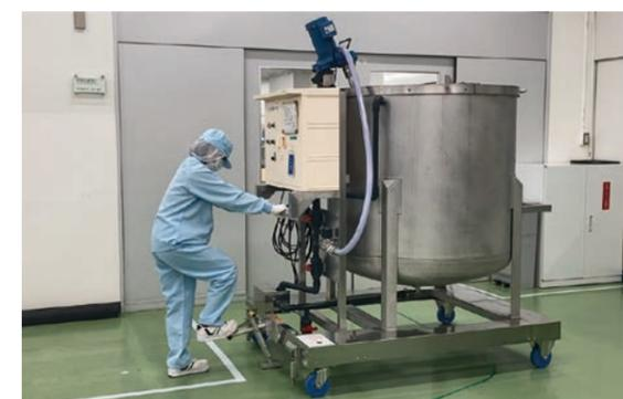
The "Helpful Pedal", which won the special award at the *Karakuri Kaizen* Exhibition (A tool that uses the principle of leverage to help transport mobile one ton tank for reagent preparation)
