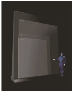
10.5-generation substrate glass
