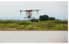
Direct-seeding cultivation on waterfilled rice paddies using a drone
