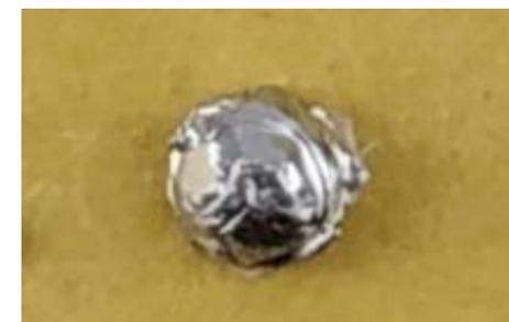
**Palladium extracted using metal adsorbent**
