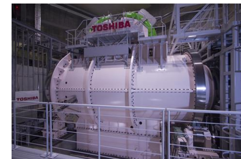
Superconducting rotating gantry: contributing to precision medicine
