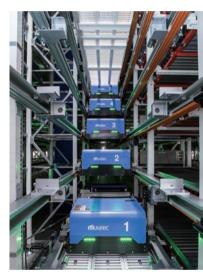
Uni-Shuttle (high-speed automated storage and retrieval system)
