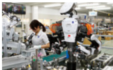
Assembly line for coin and banknote recyclers for cashiers (Saitama Factory)
