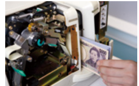
Sealing technique that bundles 100 bank notes of the same denomination with a strip of paper
