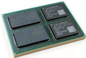
A test processor designed for V93000 EXA Scale test system
