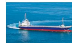
Hybrid Cargo Ship "Utashima" equipped with lithium-ion batteries
