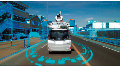
Real Dimension vehicle-mounted 3D road condition surveying system
