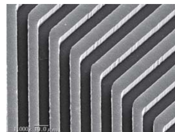
Copper wiring formed from the new seed film (thickness: 8 μm) Diagonal wiring L/S: 10/10 μm, vertical wiring L/S: 8/8 μm
