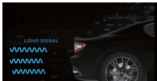
The NIR wavelengths of LiDAR signals are absorbed by the carbon black pigment of automotive coatings, significantly hindering signal response.
