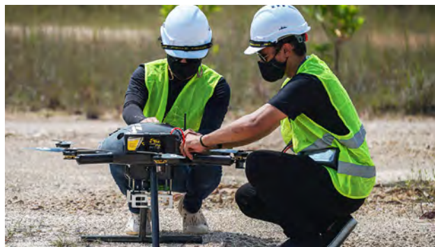
1,000-hour flight test Conducted 1,000 hours of continuous flight testing in Malaysia in cooperation with Aerodyne Japan. Performance and durability of the entire drone system was evaluated for Level 4 flight.
