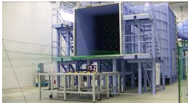
Wind Tunnel Testing Study the optimal flight of drones in terms of aerodynamics to improve its safety
