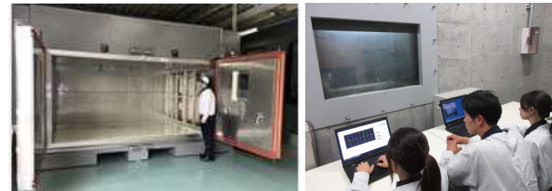
Capable of performing various safety tests for secondary batteries compliant with United Nations regulations and other standards
