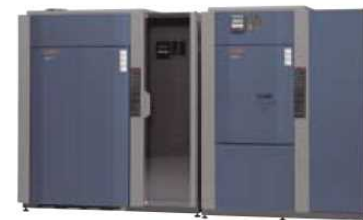
Burn-In chamber for semiconductor inspection
