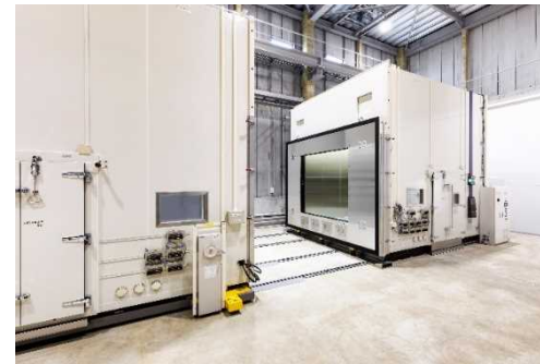
Temperature (& Humidity) Chambers are movable so that building materials for testing can be easily changed
