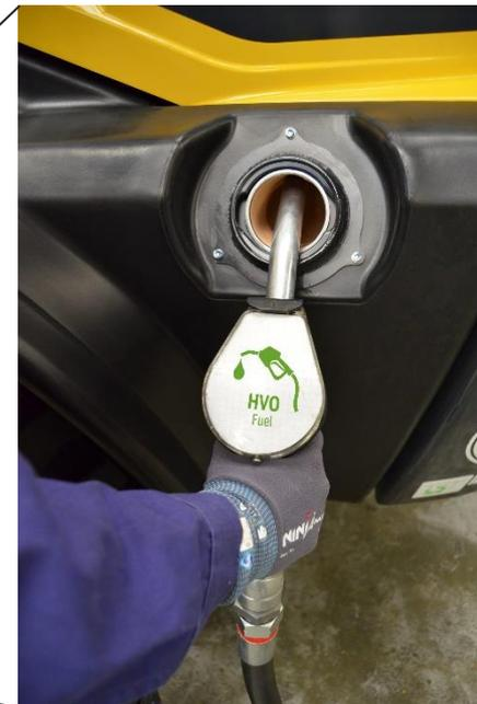
Filling a Komatsu machine with HVO as factory-fill fuel at the KGC plant in Hannover, Germany
