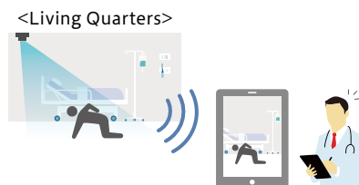
Detects falls using skeletal recognition technology and 3D cameras
