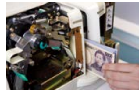
Sealing technique that bundles 100 banknotes of the same denomination with a strip of paper
