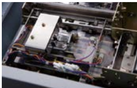
Bill validator reading banknotes to instantaneously identify denominations and verify authenticity
