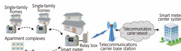
Configuration of the gas smart meter system
