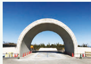
Completed development pouring for renewed lining technology
