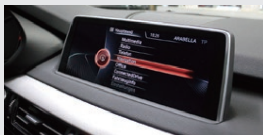
A cluster panel with an LCD using a polarizer
