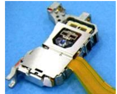
Newly developed DVD optical pickup
