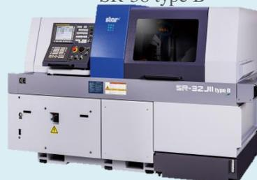
CNC Swiss Type Automatic Lathe
