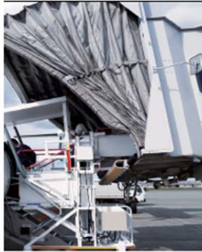
Passenger boarding bridge adaptor for turbo-prop aircraft
