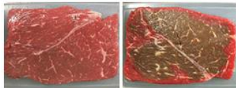
Beef discoloration test - after three days of storage (showing the underside of the meat) (Left) Fresh Master (Right) Unicharm's meat paper product
