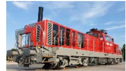
Hybrid locomotive complying with European standards(Drive system combining SCiB™ and PMSM)
