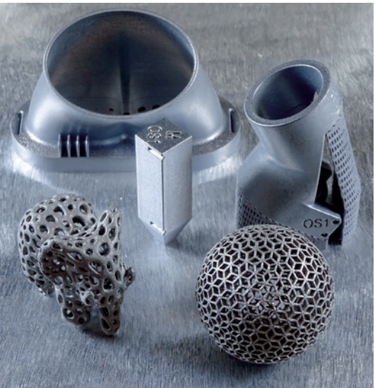
Model objects made by metal 3D printing
