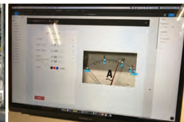
Images of meters are remotely checked and automatically converted into numerical data
