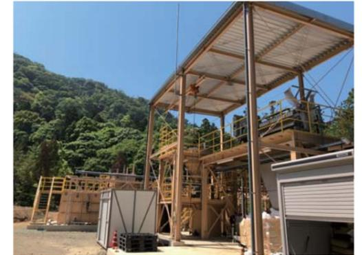
New acidic water treatment equipment has started operations. (Udo Mine)
