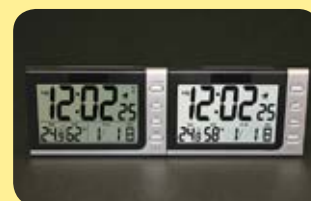
Reflective LCD that uses light diffusion film (right)
