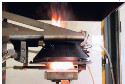
Standard PVC Plate Ignites and Burns after 35 Seconds
