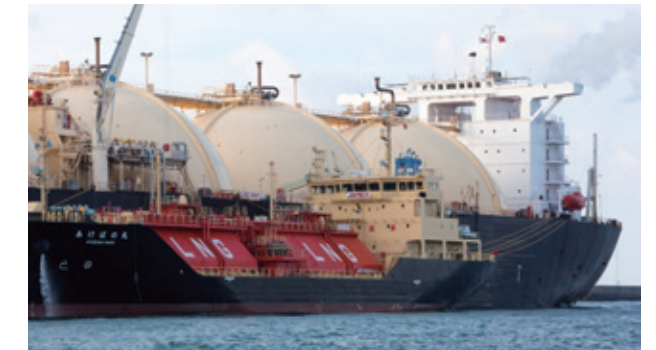
LNG being transferred from an ocean-going LNG vessel (background) to the domestic LNG vessel Akebono Maru (foreground)
