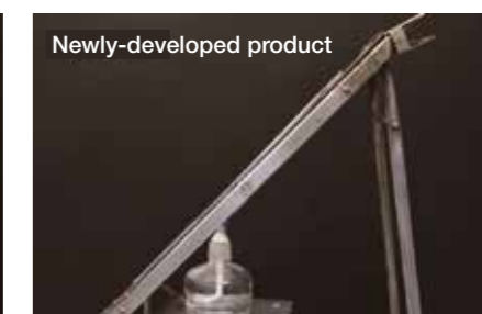
Smoke test with heating from alcohol lamp
