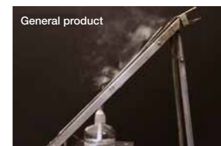
Smoke test with heating from alcohol lamp
